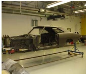
As of now, the Dodge Charger is in the shop at Clover Park Technical College and has been completely disassembled and various components are currently being prepared for repair and rebuilding. The body has been stripped to bare metal by [Strip Masters](#), a local sandblasting company and metal work on the body has
